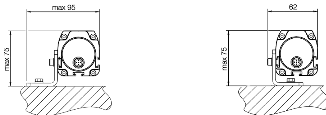
Figure 46 – Dimensions of the angled fixing bracket with a profile
